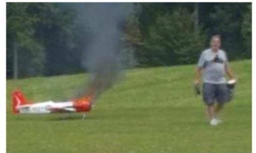
The plane had no visible damage and was placed on the runway for another flight. However, the motor sounded odd and did not have its normal power. After a few short circuits around the field, the pilot landed, and smoke was issuing from the plane. Within seconds of removing the hatch, the motor compartment of the plane was engulfed in flames.
