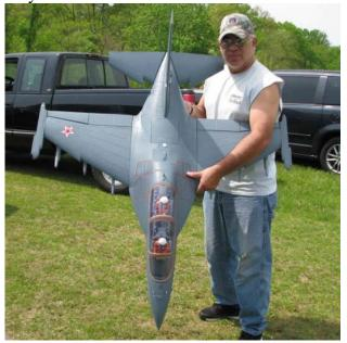
Noel Garcia brought out his new YAK-130 jet. It has a 90 mm fan and uses a 6S, 50C, 5200 mah LiPO battery. It was not maidened that day.
