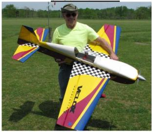
Yours truly showed a new Velox Revolution 2 that I ordered from a hobby shop in Greece. The model has a 68" wingspan and is powered by a Saito 125 4-stroke. Nate Smallwood did the test flight and when I took the sticks I found it to handle very well.
